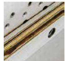
Some rail profiles have dried lubricant present
