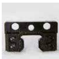
End seal in good condition
